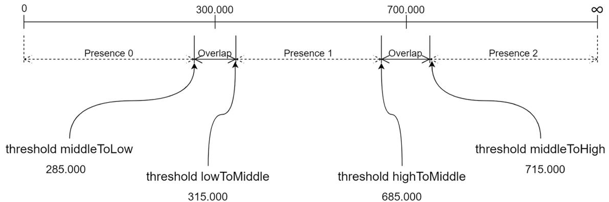
When calibrating (full process explained in the next part) a good rule of thumb in defining the thresholds is to stand where we would like the sensors to “detect” us. Take a small step forward (lowToMiddle) and a small step backwards (middleToLow). That gives us pretty accurate values keeping around a 10% margin.
