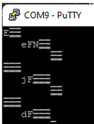
In this case type the following command: “enableTextMode” or “getSerialNumber” and hit enter. Any command can be executed like this from PuTTY, we should see an immediate change in the output.
