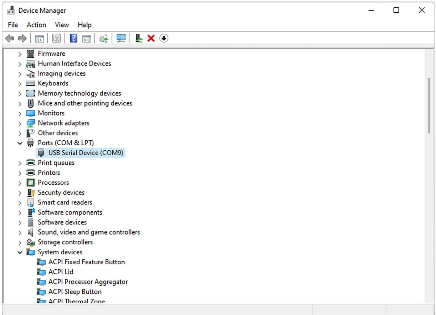
When the correct port is found we can open a program like PuTTY (for Windows, Linux & Mac) to test our serial communication. We insert the COM port and set the Baud rate of 115200 as our speed.
